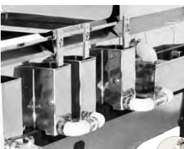
High temperature foodgrade SILICONE interconnections
